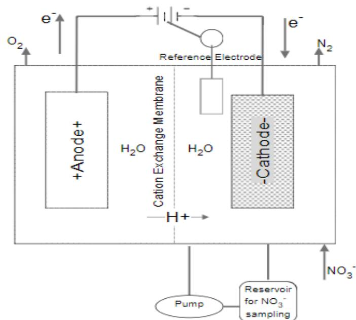
The design in Figure 1 consists of a two-cell reactor: the cathode cell and the anode cell. The electrode (cathode), where nitrate-reducing microbes are immobilized, serves as the direct electron donor to the microbes.<sup>1</sup> With a continual flow of hydrogen ions from the anode chamber and electrons from the cathode, microorganisms will reduce nitrate to harmless nitrogen gas. The reduction of nitrate in the cathode cell, on the cathode, follows the stoichiometric reactions listed below:
